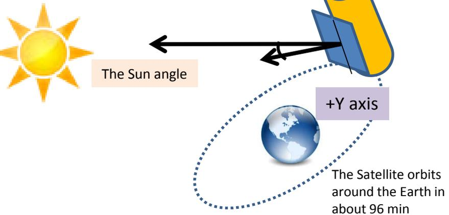
The nominal angle between satellite +Y axis and the Sun angle is within  $\pm 30$  degrees.
