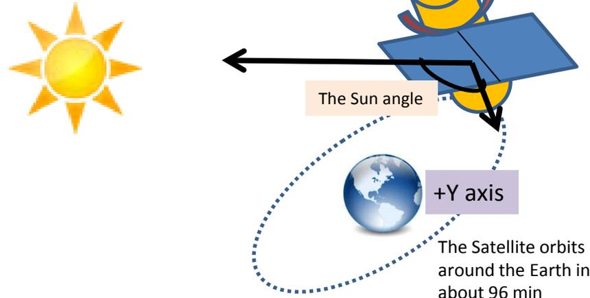
The IRU estimated error value continues, and ASTRO-H began to rotate along Z axis about 21.7 degree/hour slowly. The Sun angle at a time of the last telemetry reception at MGN was about 123 degrees.
