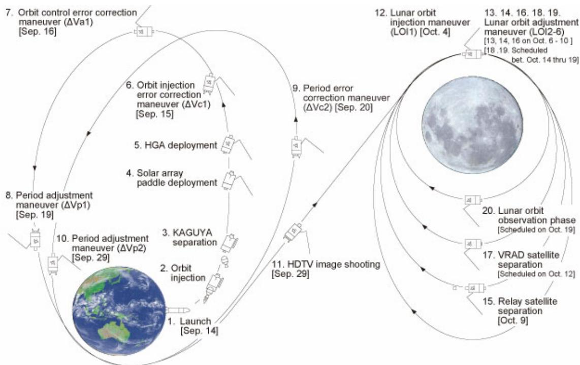
\* Lunar orbit adjustment maneuver (LOI4): orbit control to lower the KAGUYA's altitude in the injected lunar orbit (16 in the above figure)
