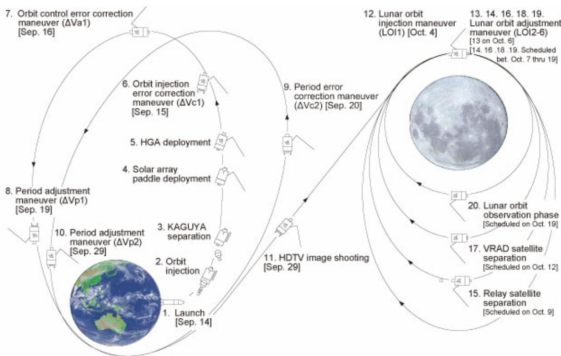
\* Lunar orbit adjustment maneuver (LOI3): orbit control to lower the KAGUYA’s altitude in the injected lunar orbit (14 in the above figure)
