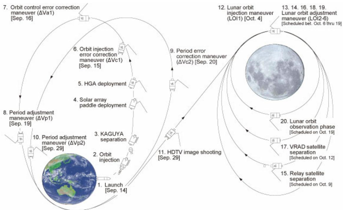
\* Lunar orbit adjustment maneuver (LOI2): orbit control to lower the KAGUYA's altitude in the injected lunar orbit (13 in the above figure)
