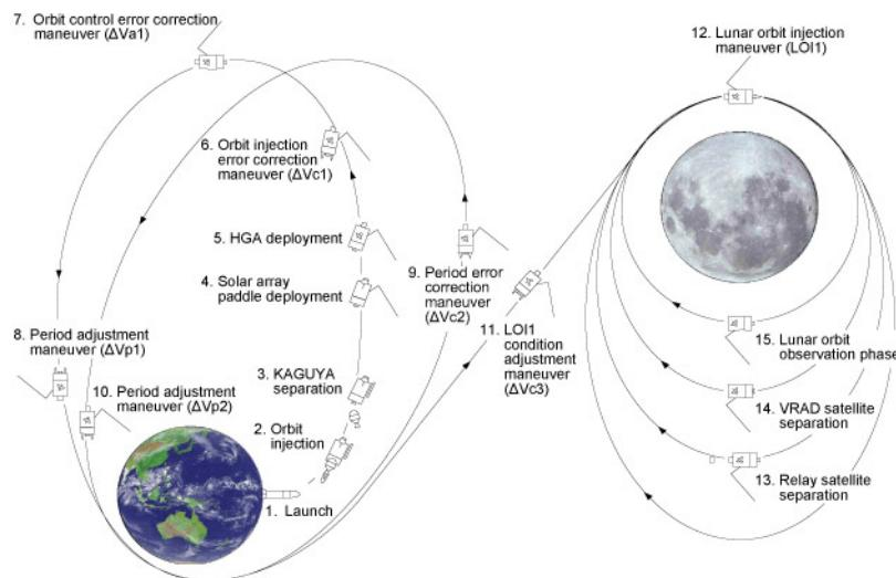
\* Orbit control error correction maneuver: orbit control to correct errors with  $\Delta V_{c1}$  orbit control
