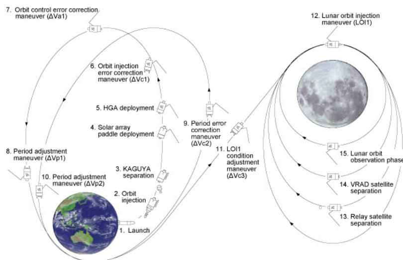
\* Orbit injection error correction maneuver: orbit control maneuver to correct errors with the KAGUYA orbit injected by the H-IIA launch vehicle and to change the KAGUYA’s orbit plan (6 in the above figure)
