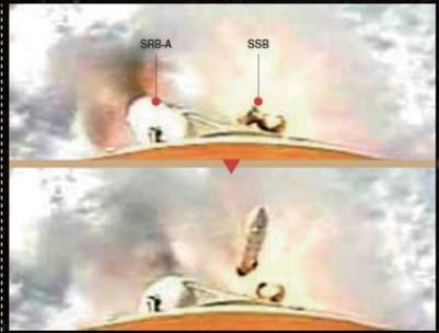
H-IIA F6 rocket immediately following launch. After separation of the solid strap-on booster (SSB; right), the vehicle failed to jettison one of its two solid rocket boosters (SRB-A; left). The launch vehicle was subsequently destroyed via a command from the ground, as it was unable to gain planned altitude owing to the jettison failure.
