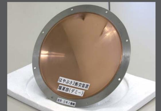
The impactor made of pure copper (photograph of a dummy model)
