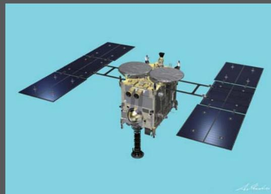
Two large discs that feature on the upper-exterior of Hayabusa2 are an X-band high-gain antenna (left) and a Ka-band high-gain antenna (right) (computer graphic image)
