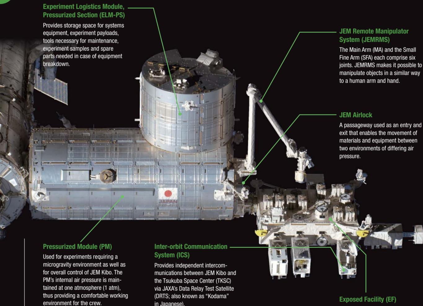
**Experiment Logistics Module, Pressurized Section (ELM-PS)**
