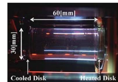
A liquid bridge of silicon oil formed between two disks of differing temperature
