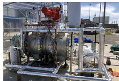
Testing state of the large valve for liquid hydrogen
