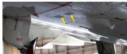
At the position with the yellow arrows, JAXA's riblet (longitudinal groove structure to reduce surface friction resistance) was processed on the aircraft. We conducted flight demonstration experiments in cooperation with the respective companies.
