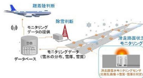
Technology system for detecting snow and ice on the runway (image)
