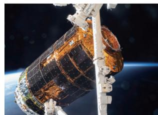
Cargo transporter "KOUNOTORI" No.9 gripped by the ISS robotic arm
